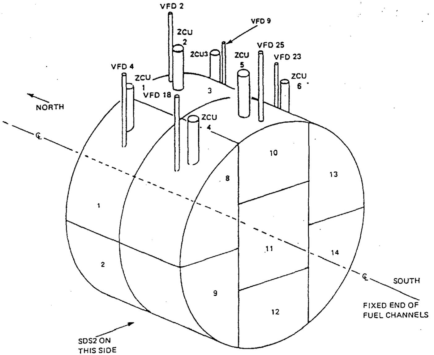
FIGURE 3.8-1 RELATION OF ZONE CONTROL UNITS (ZCU) TO THE FOURTEEN ZONES AND THE REACTOR ZONE CONTROL DETECTOR ASSEMBLIES VFD 2, 4, 9, 18, 23, 25
