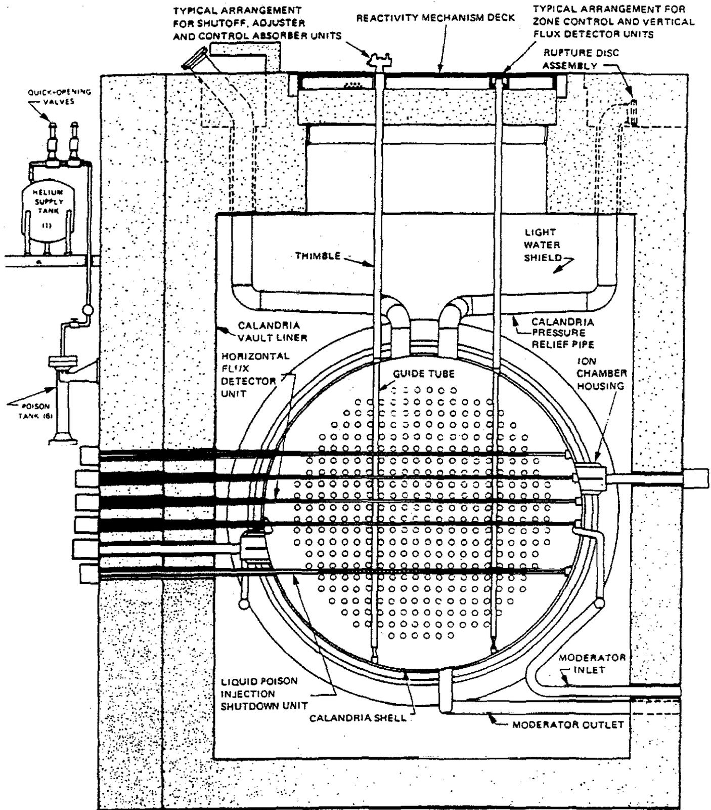
FIGURE 4.1.1-2 REACTOR LAYOUT - ELEVATION
