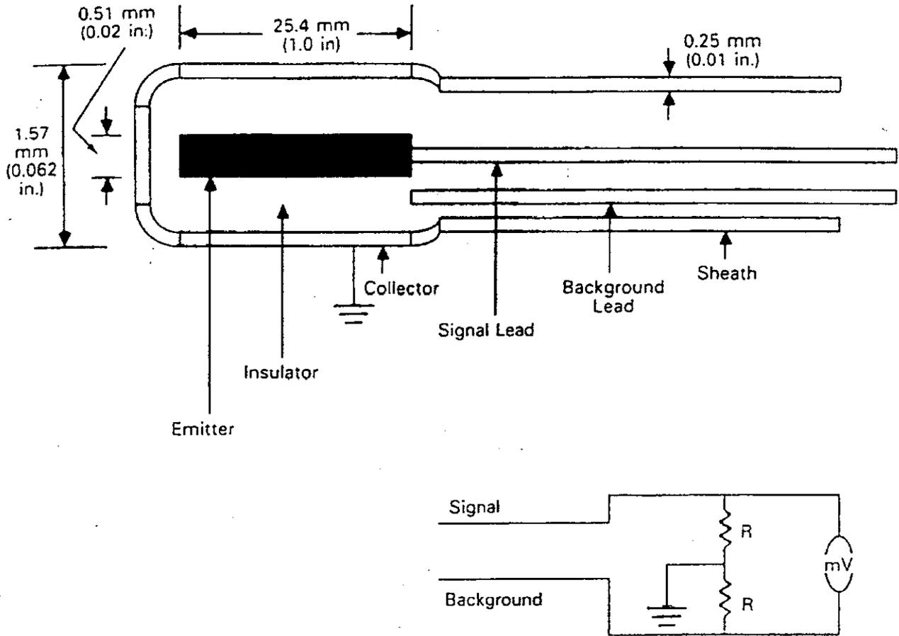
Fig. 1. Schematic of SPND with automatic background subtraction.
