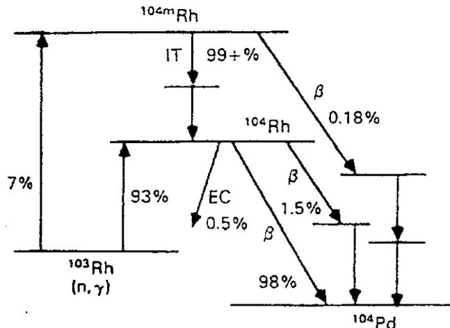
Fig. 2. Decay scheme of rhodium relevant to SPND.
