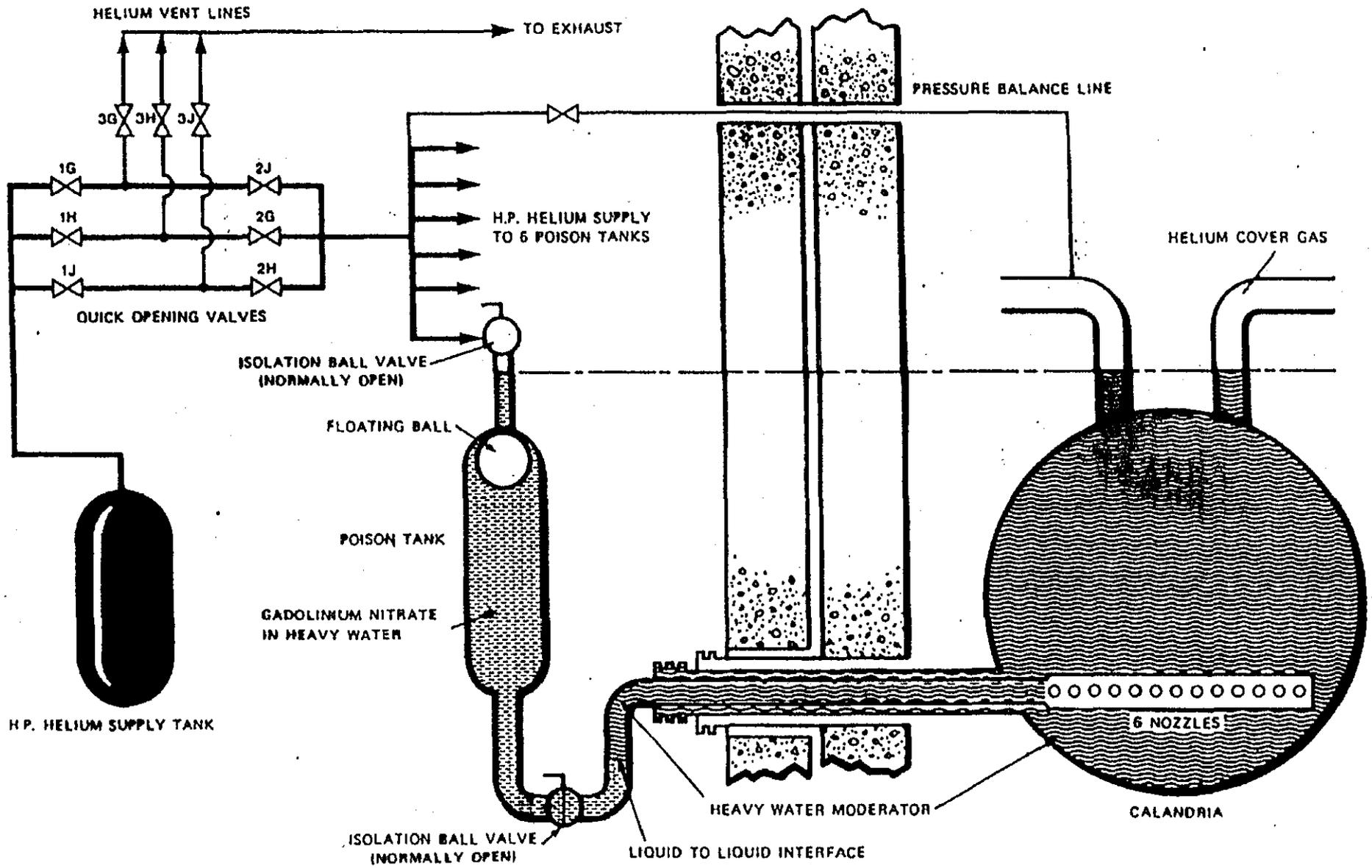
FIGURE 6.5 - 3 SHUTDOWN SYSTEM NO. 2
